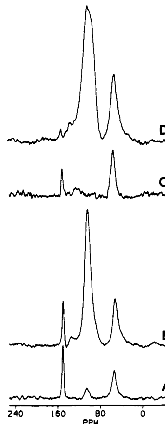
Figure 4. 26.5-MHz ^{15}\text{N} CP/MAS spectra. (A) Interrupted-decoupling spectrum ( \tau = 2 ms; interrupt time = 100 \mu\text{s} ; t_d = 6 s) of MDI-based resin after heating at 300 °C. (B) Normal spectrum ( \tau = 2 ms; t_d = 6 s) of MDI-based resin after heating at 300 °C. (C) Interrupted-decoupling spectrum ( \tau = 1 ms; interrupt time = 100 \mu\text{s} ; t_d = 6 s) of MDI-based resin after heating at 340 °C. (D) Normal spectrum ( \tau = 1 ms; t_d = 6 s) of MDI-based resin after heating at 340 °C.
